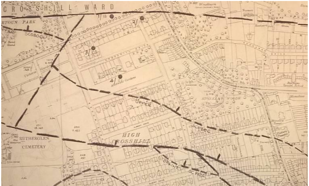
The map above shows the location of four shafts of the Low Crosshill colliery, along and to the south of Roger Drive. The map also shows, as dotted lines, where the coal seams outcrop at ground surface. (Reproduced by permission of the British Geological Survey [2018]).
