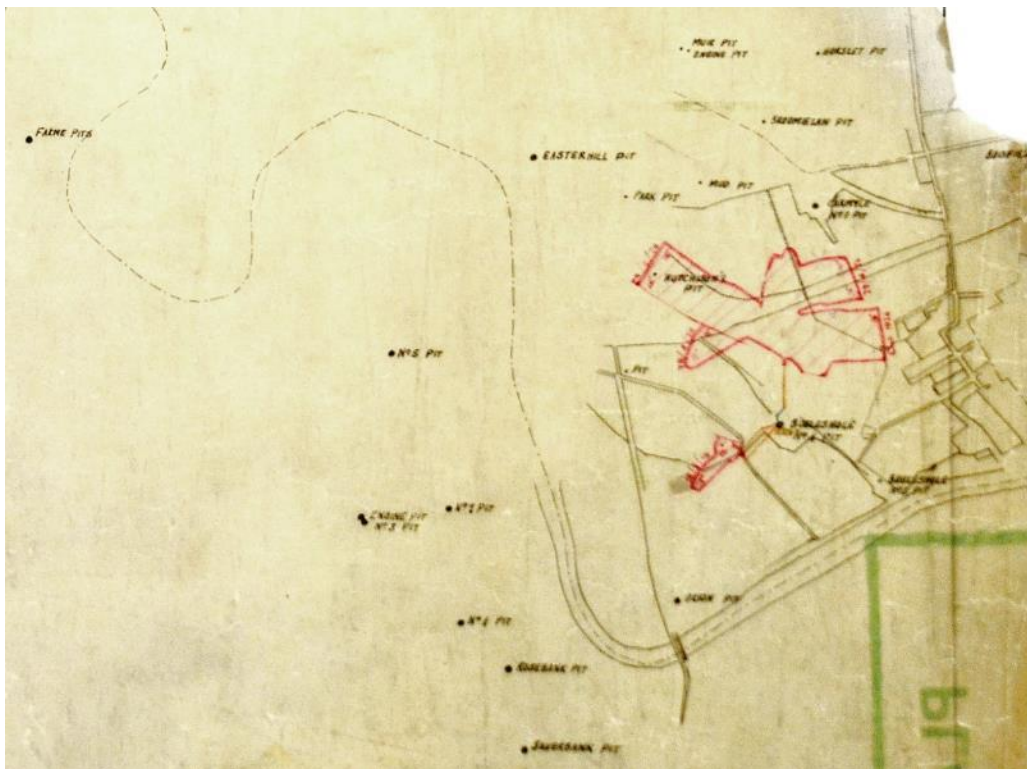
Map showing the location of Rosebank Pit, second up from the bottom of the map (Reproduced by permission of the National Records of Scotland, Ref 67). This shaft was located and grouted in 1981 (Ref 22).
